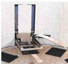
Figure 31 Both transport locks refitted
