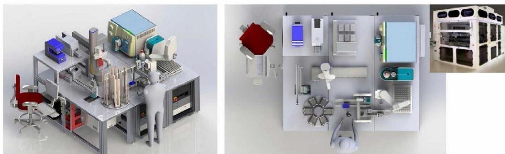
Figure 2. Scheme of automated HT peptide-MS workflow. The full enclosure in a biological safety cabinet (S-CEL4000 with HEPA filter) is shown in insert.
