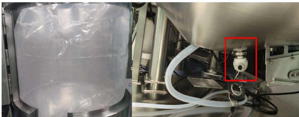
Figure 2 On the left the tank bag during tank assembling, on the right tank temperature probe detail.
