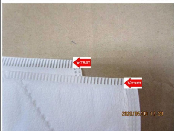
↑ 6 - Remark 1, uneven width of the edge
