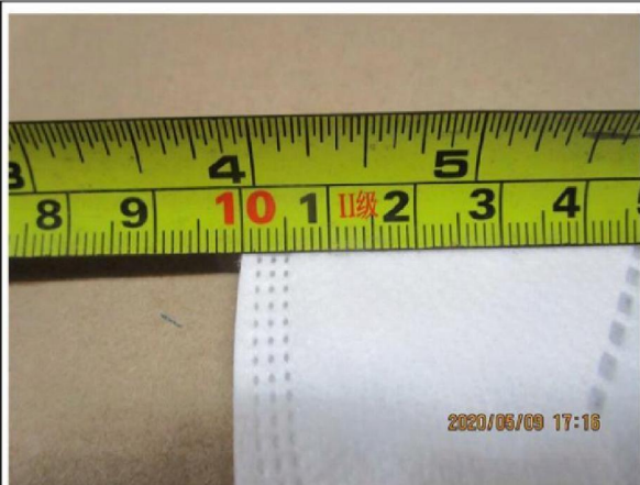
↑ 2 - Remark 1, uneven width of the edge
