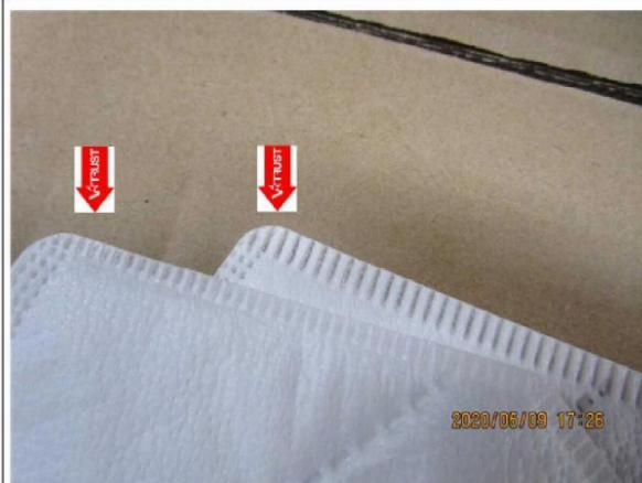
↑ 7 - Remark 1, uneven width of the edge
