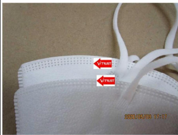
↑ 4 - Remark 1, uneven width of the edge
