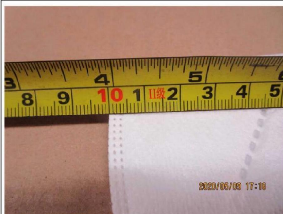
↑ 1 - Remark 1, uneven width of the edge
