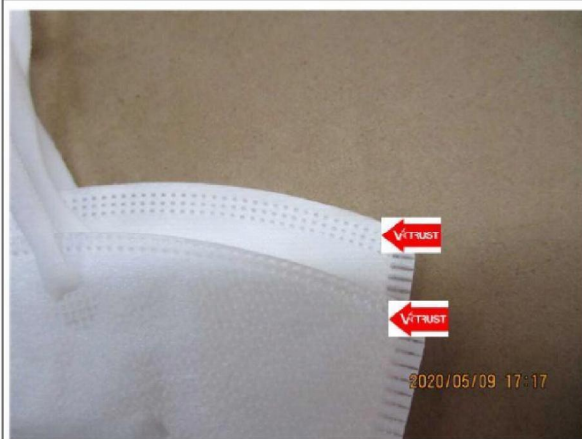
↑ 5 - Remark 1, uneven width of the edge
