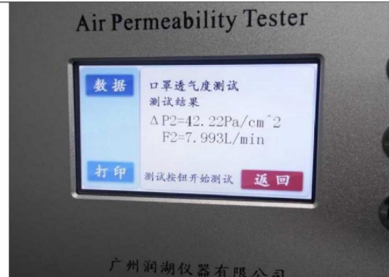
Differential pressure test (2)
