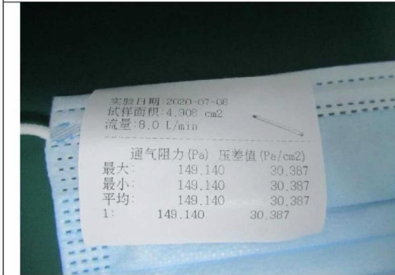
Differential pressure test
