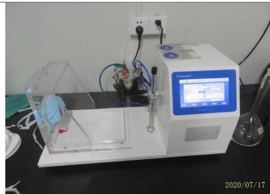
Synthetic Blood Penetration test
