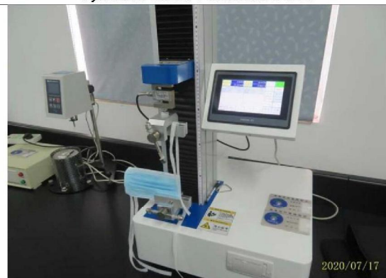
Tension test on ear loop
