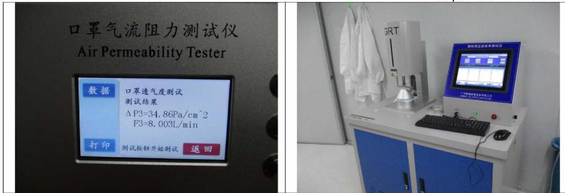
Differential pressure test
