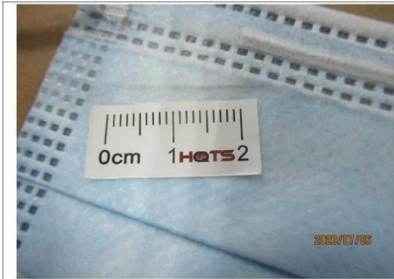
Defect- Fold mark on surface-mi
