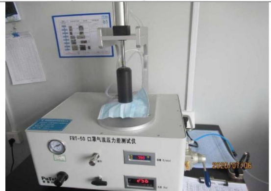
35 differential pressure test
