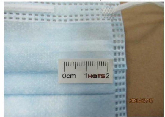
Defect- Fold mark on surface-mi
