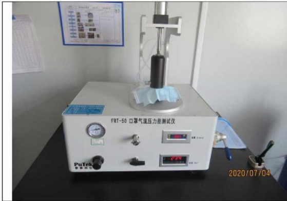
24 differential pressure test
