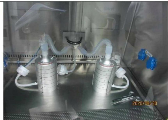
Bacterial filtration efficiency test
