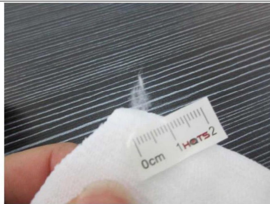
Defect- Snagging yarn(0.6cm)-ma
