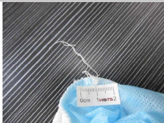
Defect- uncut thread (3.5cm)-mi
