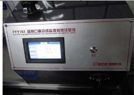
Synthetic blood penetration test
