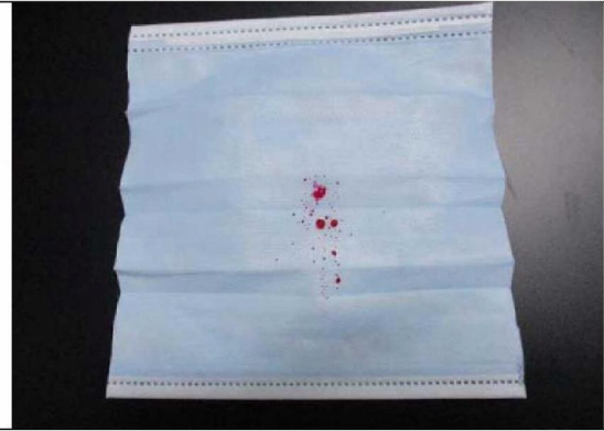
Synthetic blood penetration test
