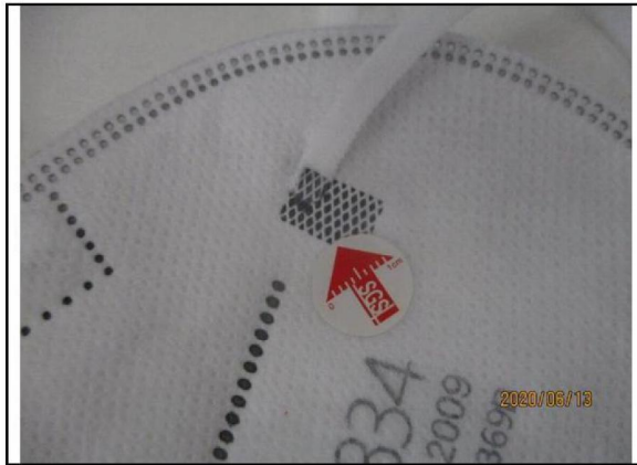
2.4 poor connection of ear loop end-minor.JPG
