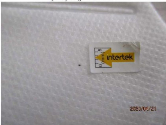
01 minor defect-dirty mark on surface
