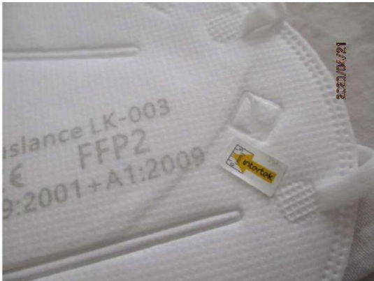
01 minor defect-wrinkle mark on surface
