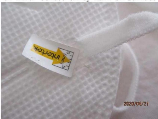
01 minor defect-dust dot on surface (2)
