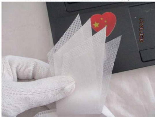
35 material layer quantity check
