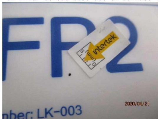
01 minor defect-print dot on polybag
