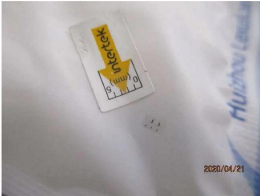
01 major defect-foreign material on polybag surface
