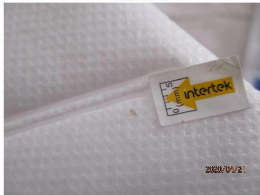
01 minor defect-dust dot on surface (1)
