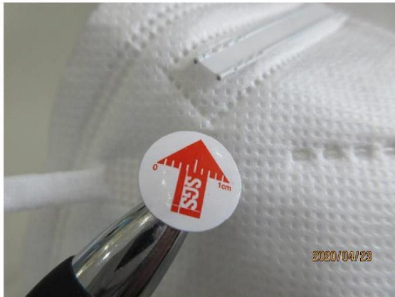
Poor heat bonding at nose clip –major
