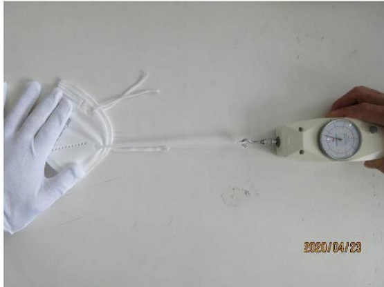
(39). strap pull test-10N,10S
