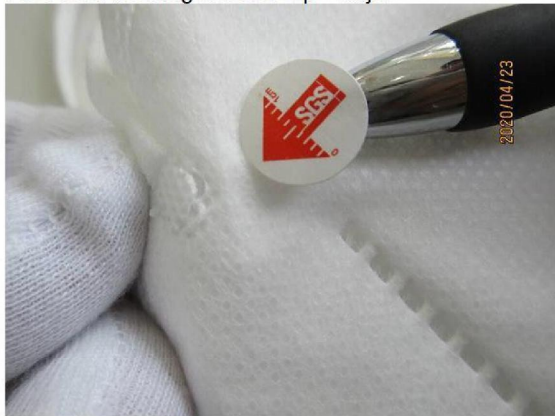
Poor heat bonding at strap – major
