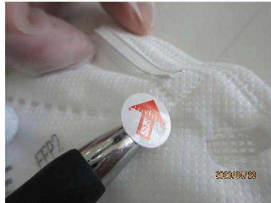
Poor heat bonding at nose clip –major
