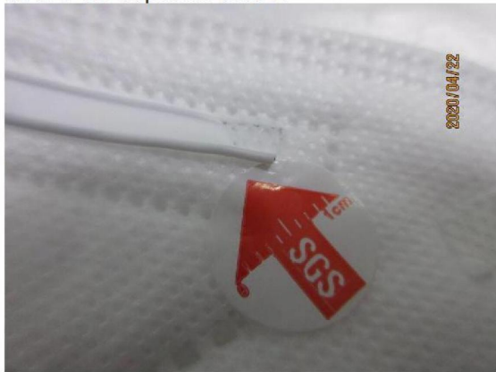
05 major-poor heat bonding.JPG
