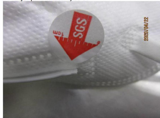
06 major-poor heat bonding.JPG
