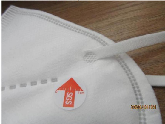
21 minor poor assembly. JPG
