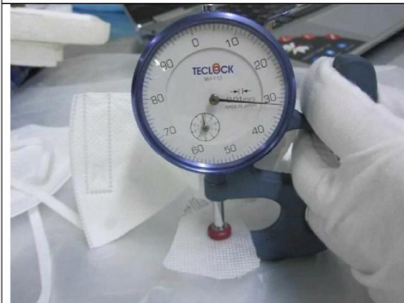
1 st layer non-woven cloth thickness: 0.32mm
