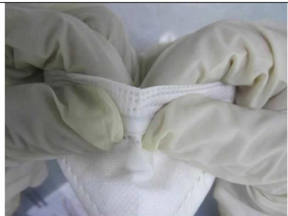
Nose clip bending life test
