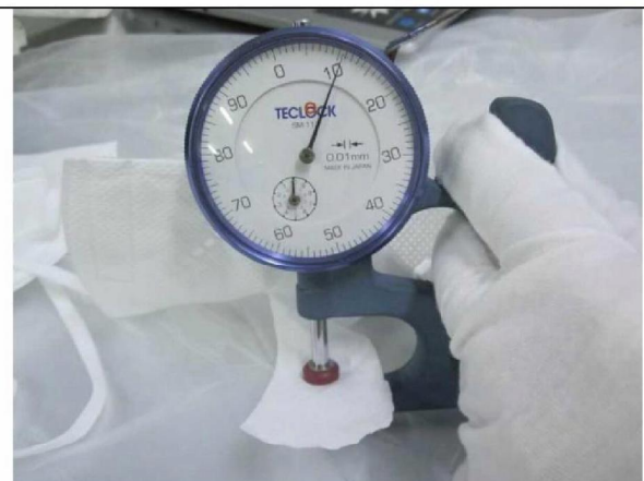
4 th layer molten cloth thickness: 0.105mm
