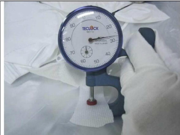
5 th layer non-woven cloth thickness-0.27mm
