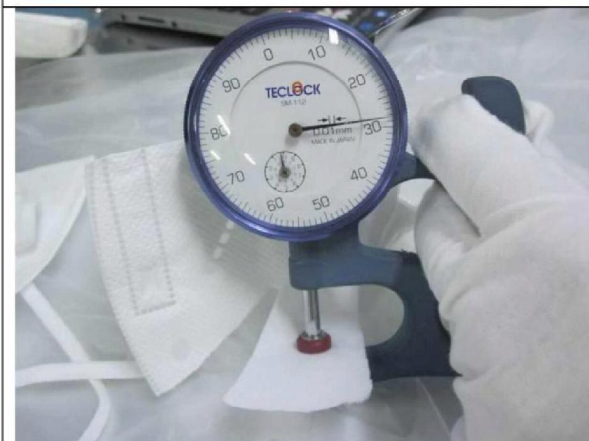
3 rd layer molten cloth thickness: 0.28mm
