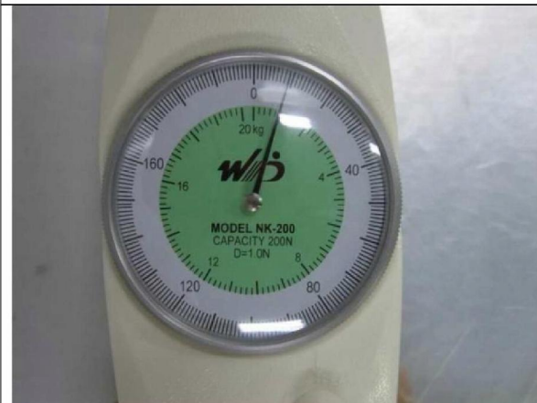
Ear strap strength test 1kgs weight(10N)
