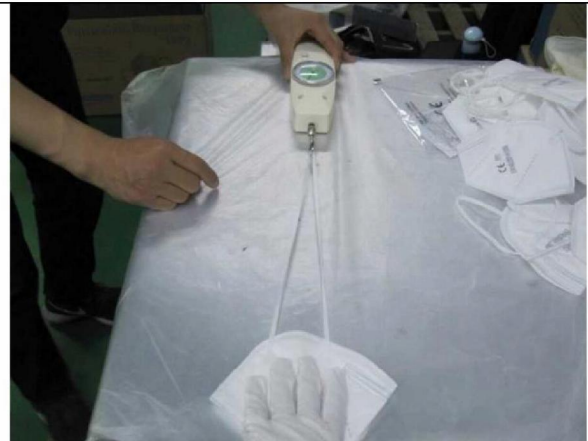
Ear strap strength test 1kgs weight(10N)
