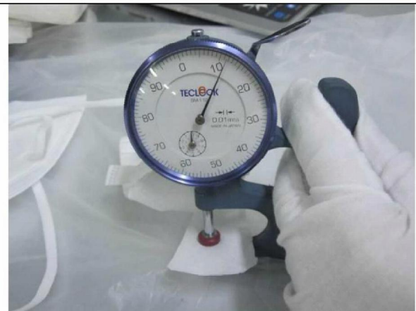
2 nd layer molten cloth thickness: 0.12mm
