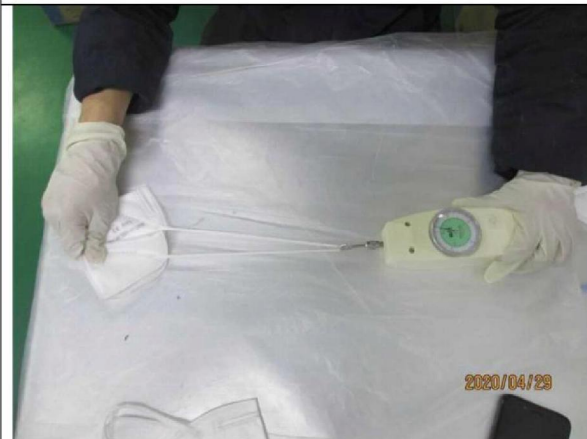
Ear strap strength test 1kgs weight(10N)
