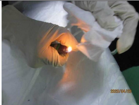
Middle layer meltblown melt , not burnt
