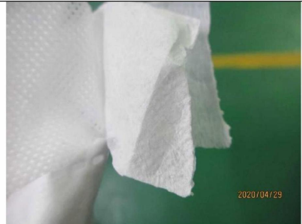
Middle layer meltblown melt , not burnt
