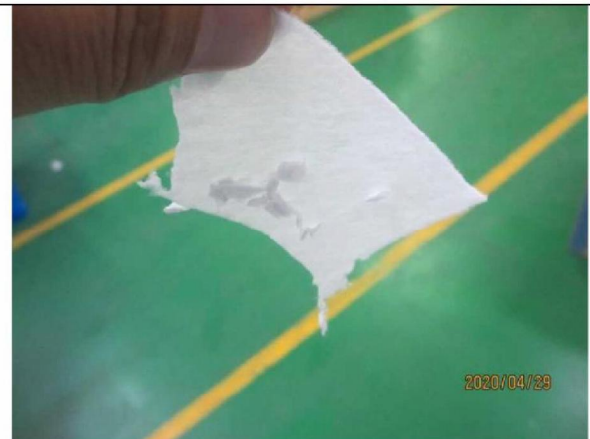
Middle layer meltblown electrostatic adsorption test
