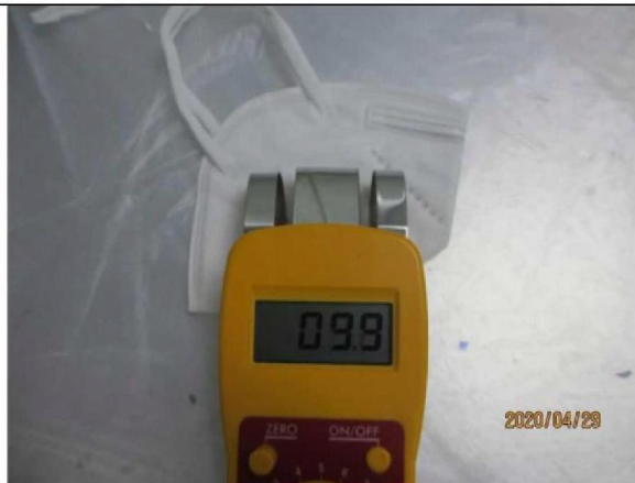
Fabric humidity check
