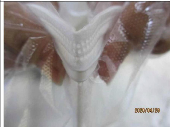
Nose clip bending life test
