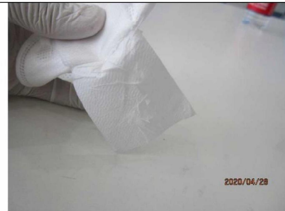
Middle layer meltblown fabric electrostatic adsorption test
