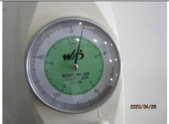
Ear strap strength test 1kgs weight 1minute, ok
