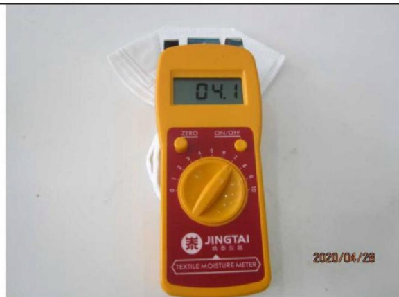
Fabric humidity check
