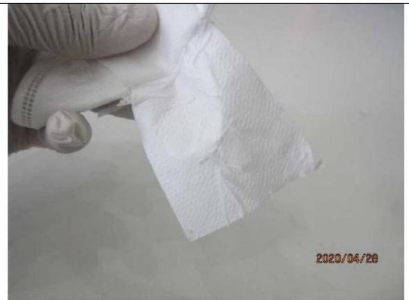
Middle layer meltblown fabric electrostatic adsorption test
