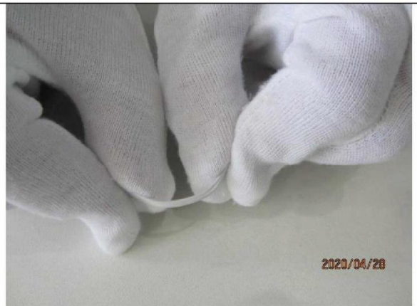
Nose clip bending life test
