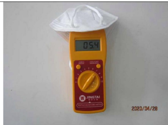
Fabric humidity check
