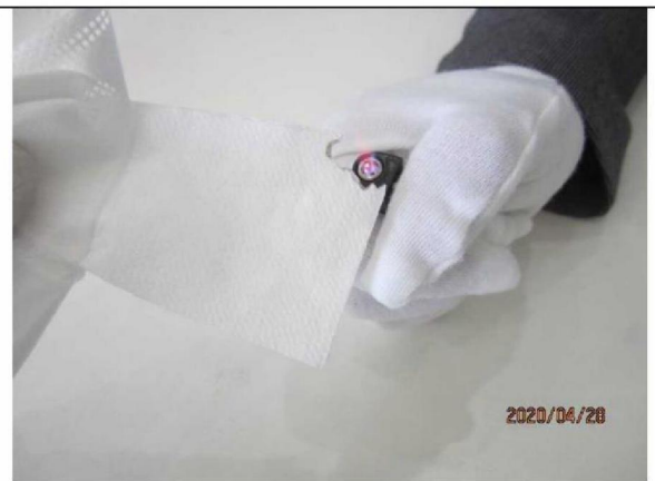
Middle layer meltblown melt , not burnt
