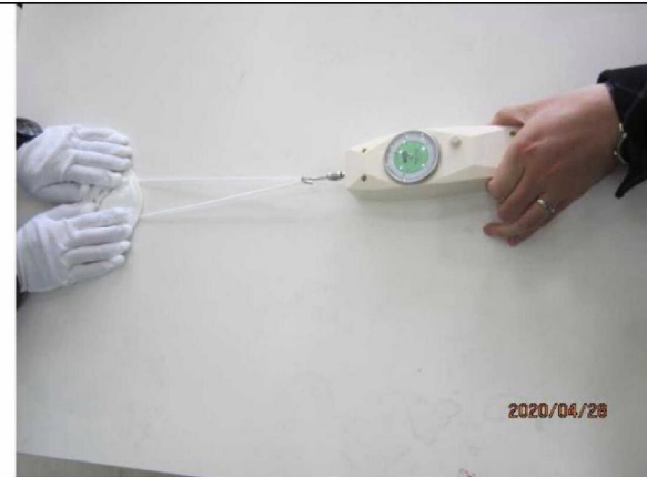
Ear strap strength test 1kgs weight
