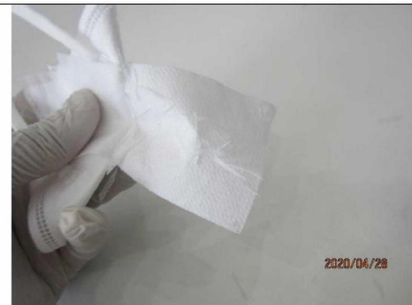
Middle layer meltblown fabric electrostatic adsorption test
