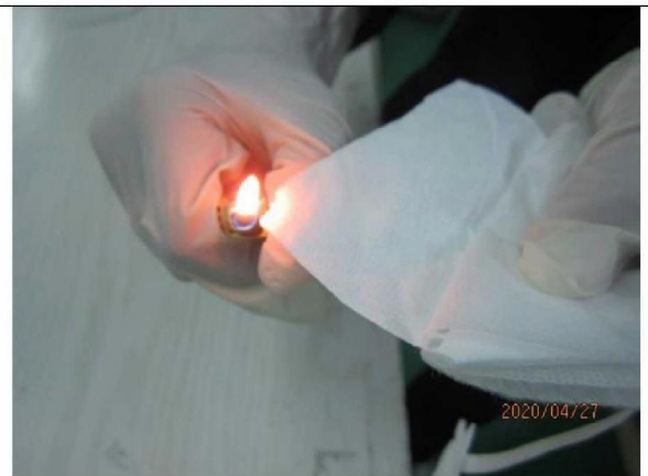
Middle layer meltblown melt , not burnt
