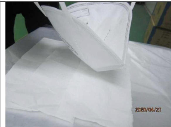
Middle layer meltblown electrostatic adsorption test
