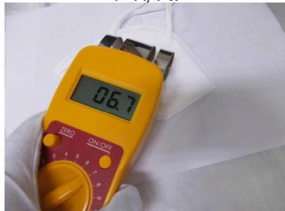
Material layer quantity check
