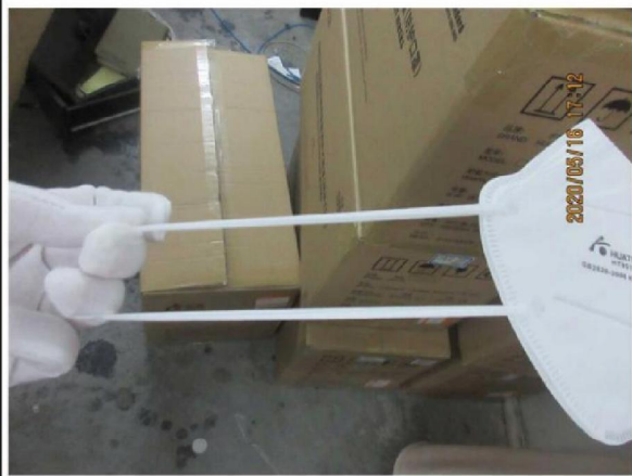
↑ 79 - Welding Strength Test
