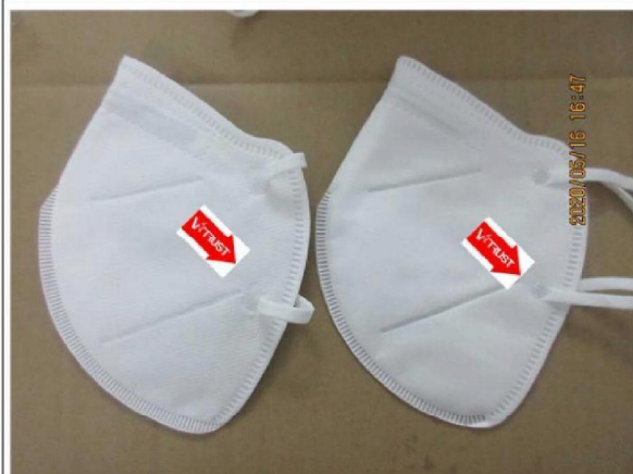
↑ 3 - Remark 4, Two lots shape of welding point were found on site. Lot A was 90%(right) and the lot B was 10%(left).
