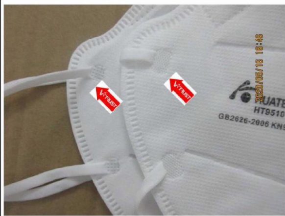
↑ 2 - Remark 4, Two lots shape of welding point were found on site. Lot A was 90%(left) and the lot B was 10%(right).
