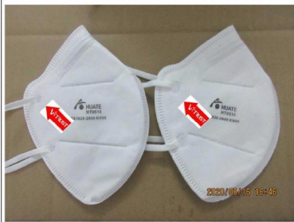
↑ 1 - Remark 4, Two lots shape of welding point were found on site. Lot A was 90%(left) and the lot B was 10%(right).
