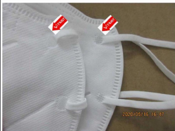
↑ 4 - Remark 4, Two lots shape of welding point were found on site. Lot A was 90%(right) and the lot B was 10%(left).
