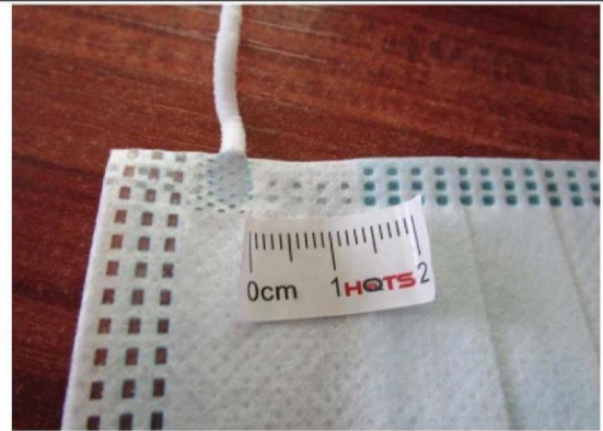
Defect-poor sealing side at unit(1cm)-mi
