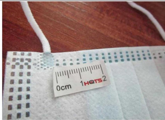
Defect-poor sealing side at unit(1cm)-mi
