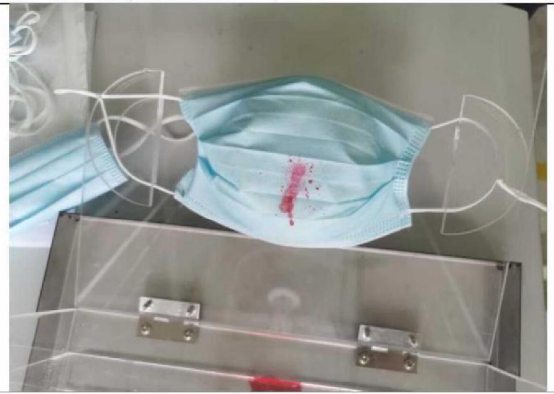
Synthetic blood penetration test
