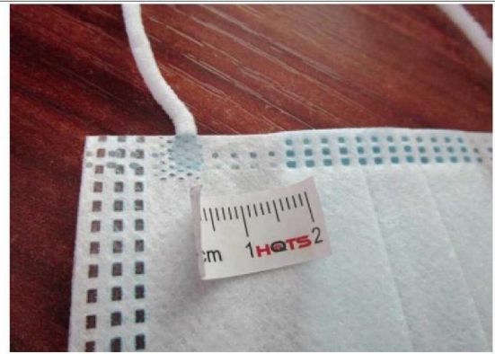
Defect-poor sealing side at unit(1cm)-mi
