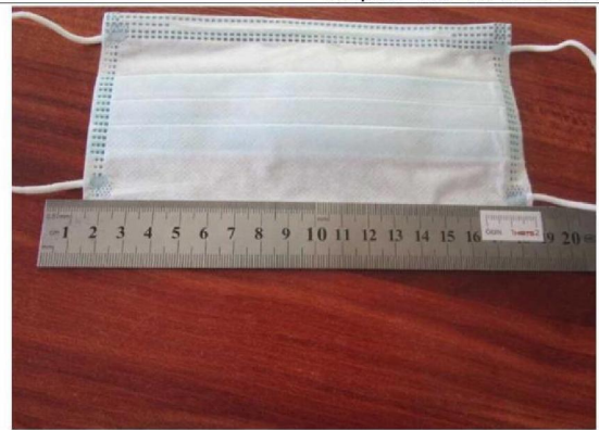
Defect-uneven position at ear loop(0.5cm)-ma
